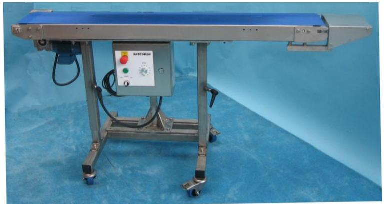
The conveyor channel has a travel facility in its design, this provides some forwards or backwards movement to offset the sealing head from centre, should the application dictate (e.g. necessary to overhang a carousel, pass through a partition, wall etc). The conveyor is variable speed and is fitted with a food grade transport belt. A tracking system eliminates belt wandering. Manufactured in stainless steel.
