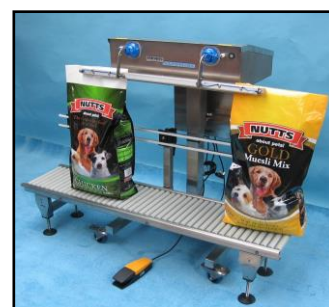
EXAMPLE Gravity roller and motorised conveyor belt conveyor designed to suit application.
