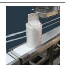
The Crimpmaster is expected to be used vertically in conjunction with a synchronised product-carrying belt conveyor system. This can be a high level system for smaller bags or a low level system to suit bulkier packs.
