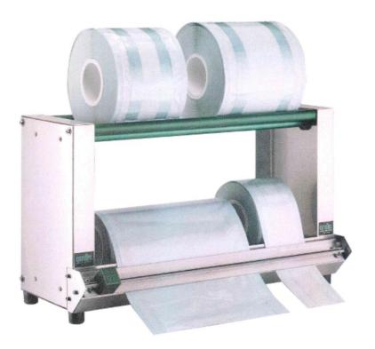
This device is offered to store and dispense a range of different widths of flat and gusseted window reels. Produced as a stainless-steel fabrication with anodised aluminium, cross rails. Designed for table and wall mounting. An integral manual trimmer allows operative control over the length of desired pouch required.
